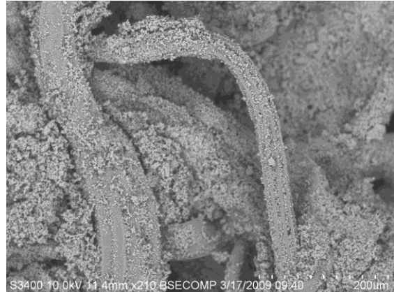
Figure 5.7. SEM image of zeolite loaded sorptive functional layer showing excessive particle loading at a loading level of 16g/ft 2 at 210X magnification
