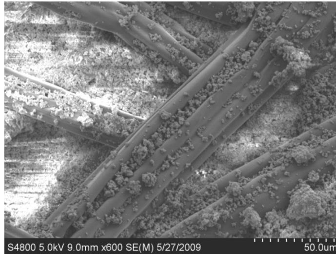
Figure 5.9. SEM image of zeolite loaded primary functional layer showing loaded grooves at a loading level of 16 g/ft 2 at magnification of 600X
