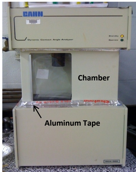
Figure 2.5. Dynamic Contact Angle Analyzer (DCA) Instrument used as a microbalance
